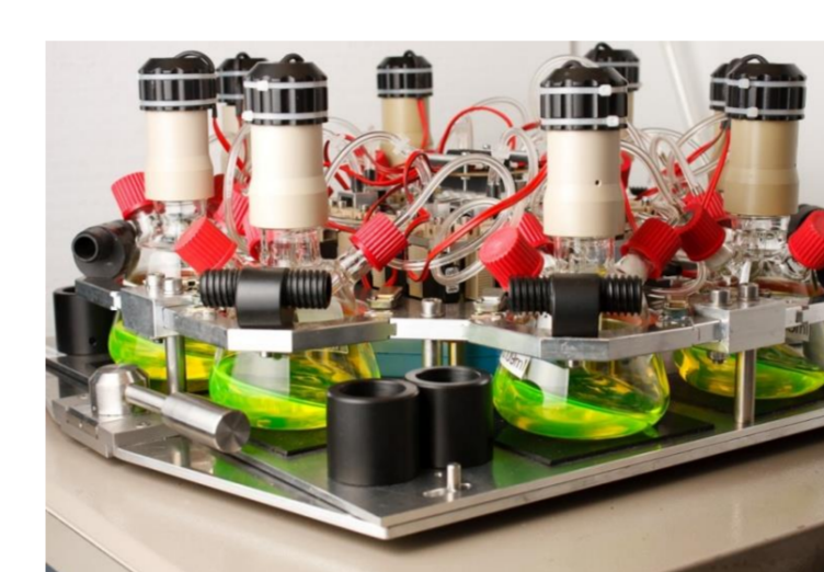
RAMOS to measure the OTR in shake flasks
