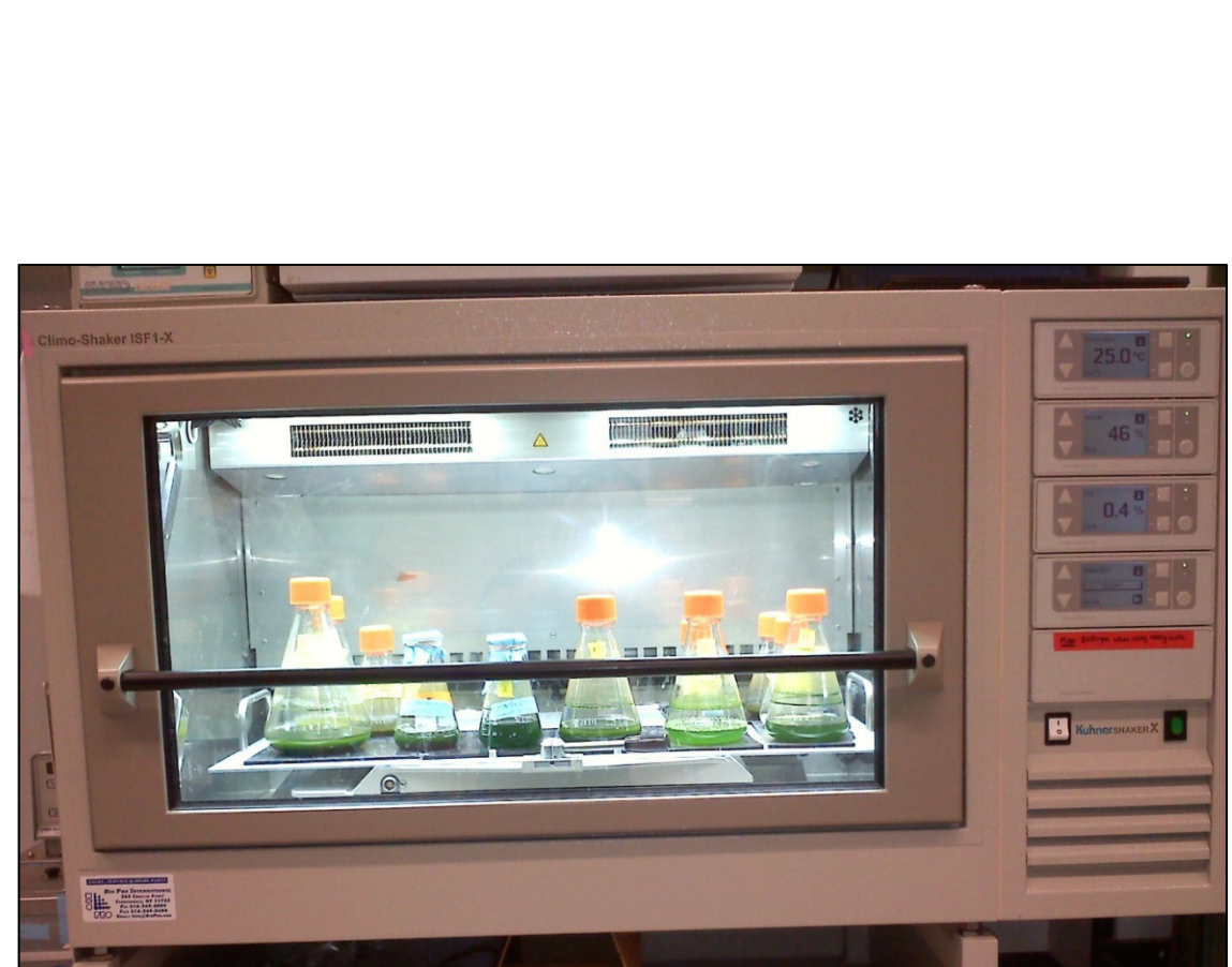
Specifically designed, climate controlled shaker for algal culture incubation (Kuhner Climo-Shaker ISF1-X),
