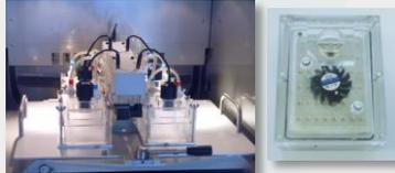
**Combination:** RAMOS technology is combined with the SFR (Presens) to measure dissolved oxygen (DO), pH, OTR and CTR in up to six flasks.
