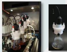
**New application:** RAMOS technology was used to test plastic components to determine their impact on the cultivation [2].
