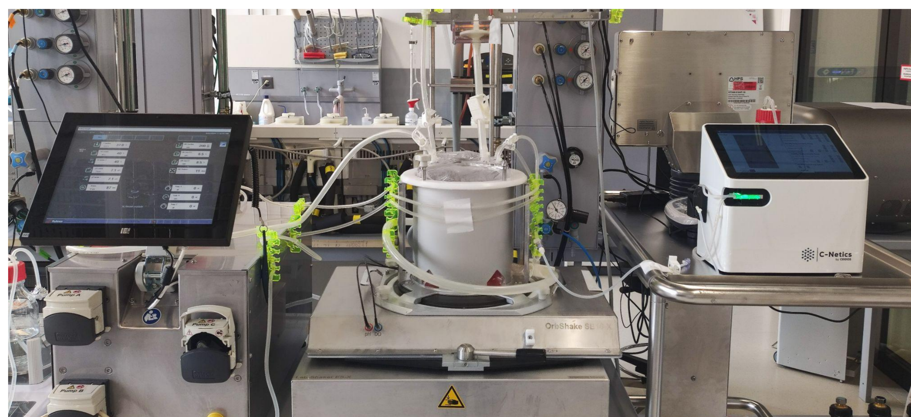
Figure 3: The C-Netics connected to SB10-X bioreactor. The samples are pumped from the bottom of the bag through the C-Netics single-use kit, where they are analyzed. The same line is used to pump cells back in the bag.
