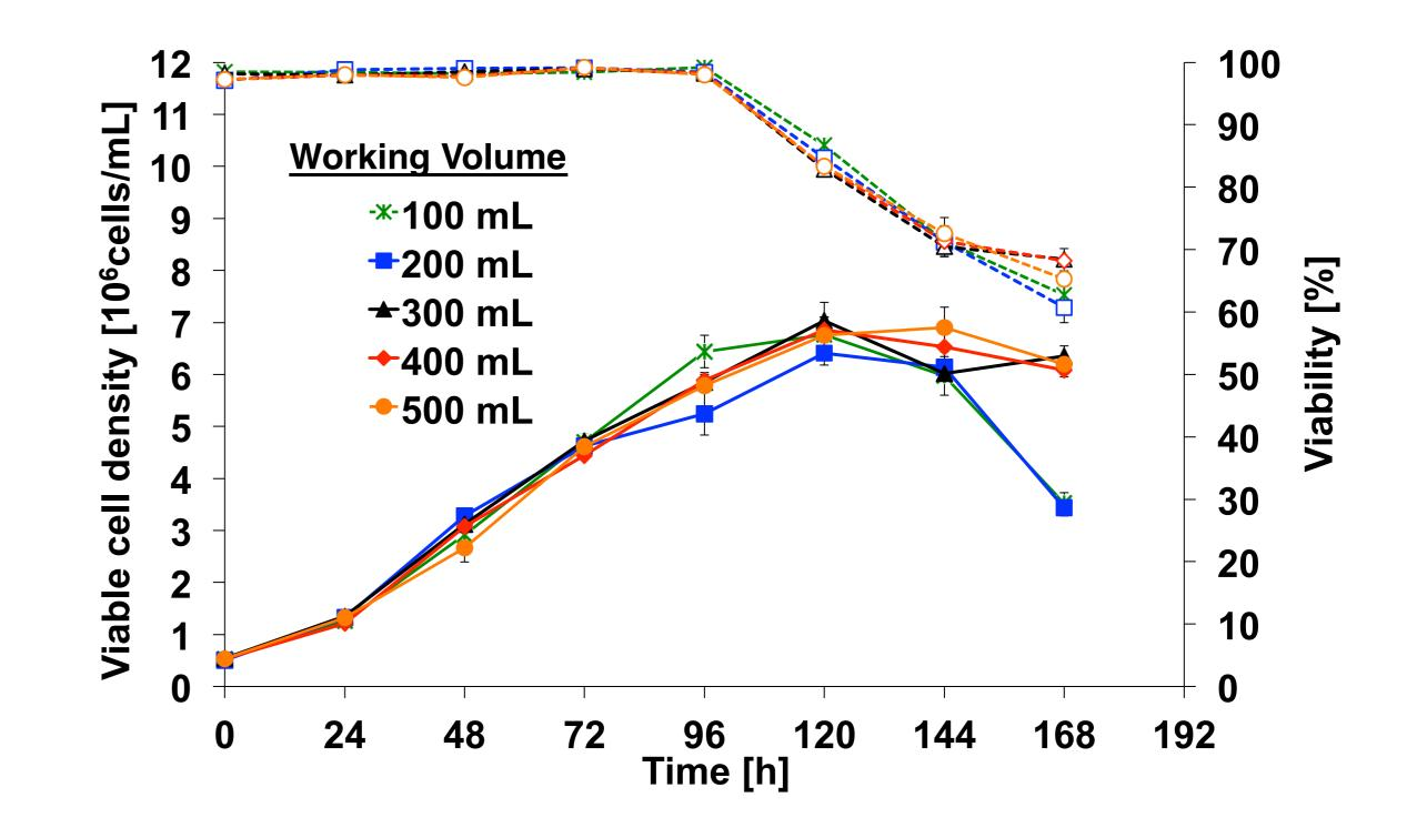
A cell growth comparison was performed with a CHO-derived cell line at different working volumes in TubeSpin<sup>®</sup> bioreactor 600 vessels. The cultures were agitated at 180 rpm with a shaking diameter of 50 mm.
