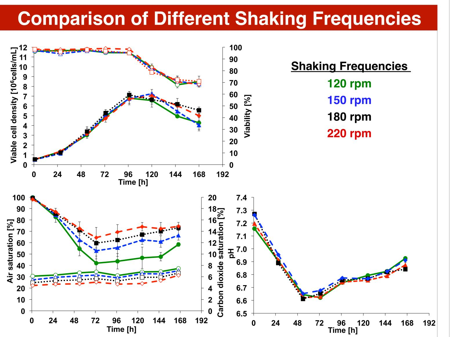
A cell growth comparison was performed by cultivating a CHO-derived cell line expressing a recombinant IgG in a TubeSpin<sup>®</sup> bioreactor 600 at different shaking frequencies as indicated. The cells were cultured at a working volume of 300 mL on a shaker platform with a shaking diameter of 50 mm. The air and  $CO_2$  saturation and the pH were measured off-line. The cell density and viability were measured by the Trypan Blue exclusion method with a hemocytometer.
